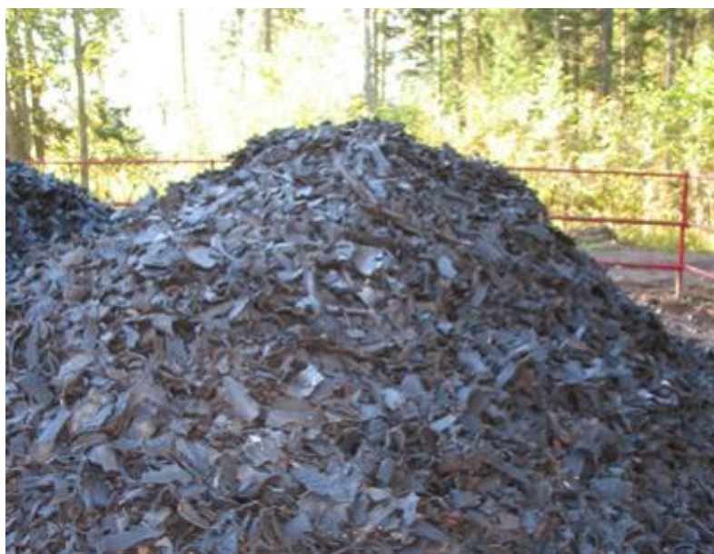
Fig 1. Chopped car tyres used for constructing the elastic paddock surface.
